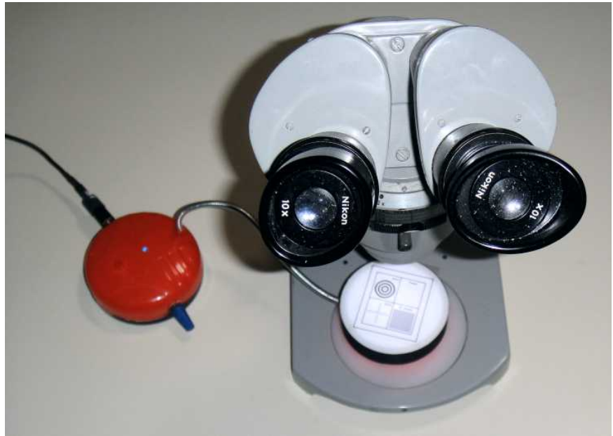
Fig. 10 – Illuminated Stage III being used with a stereo microscope.
