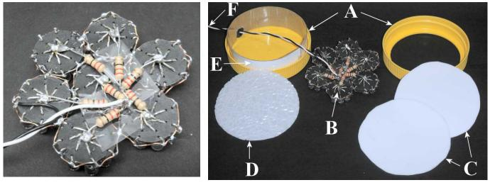
F 17 – Current limiting 22 ohm resistors. Fig. 18 – Parts for the LED illuminated stage.
