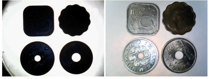
*Fig.* 7a – Back lighting only shows the silhouette. *Fig.* 7b – Low back light and full microscope LED light.
