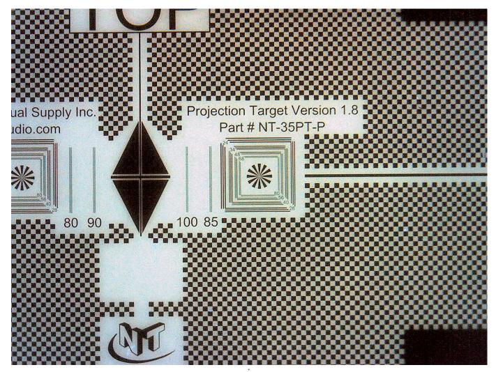
Fig. 11 - Same image as Fig. 10c enlarged further. The magnification here is 30x. Each square = 0.10 mm.
