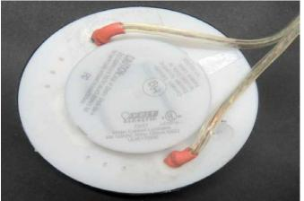
*Fig.* 5 – *Soldered power cord is insulated with heat shrink tubing. Bend flat while hot.*
