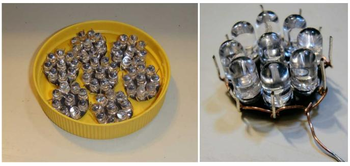
Fig. 15 – 7 LED assemblies fit in a plastic mustard cap.
