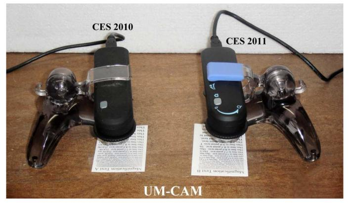
Fig. A3 – USB microscope/webcam for general use up to 45x (printed landscape). The legs have NIB magnets.
