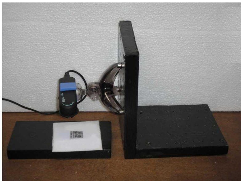
Fig. 3 – Metal covered wood “book end” stand for the UM-CAM.
