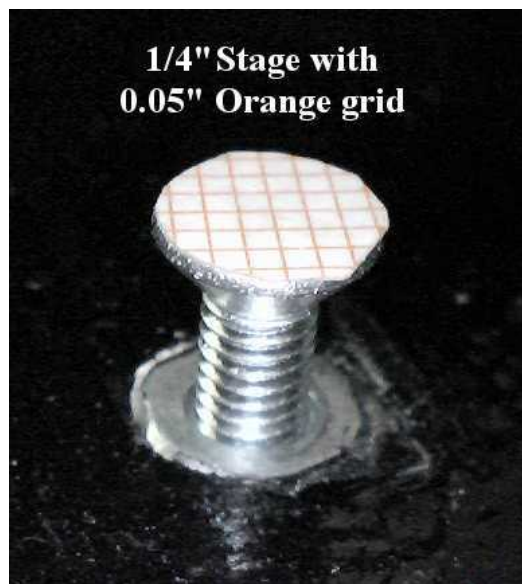
Fig. 4 – Small specimen stage with grid. UM photo.
