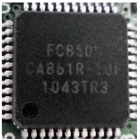
Fig. 8d – IC, 48 leads with P/N.
