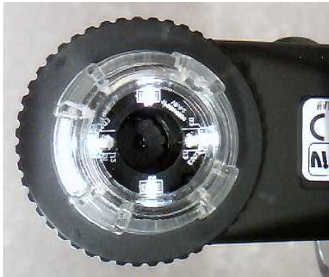
Fig. 2 – Four white LEDs light the small specimen..
