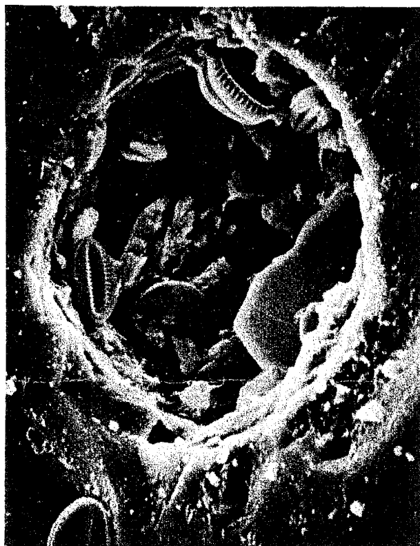
Sand Grain - Detail of Hole "A" from photo at left Hitachi Scanning Electron Microscope Model S-104a 1500X
