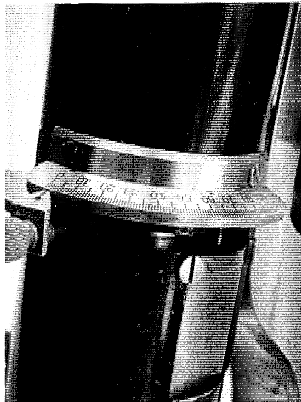
Ninety degree sector scale for the analyser. When pushed out of the optical path, the operating/index lever hangs precariously in space. Not visible higher up on the tube is the lever for the Bertrand lens iris. It is bent forward at almost 90 degrees. I thought the fragile lever had suffered a bump, but in his description of this instrument, Johanssen mentions that this was the way it was built in order to clear the Bertrand lens slider directly above.
