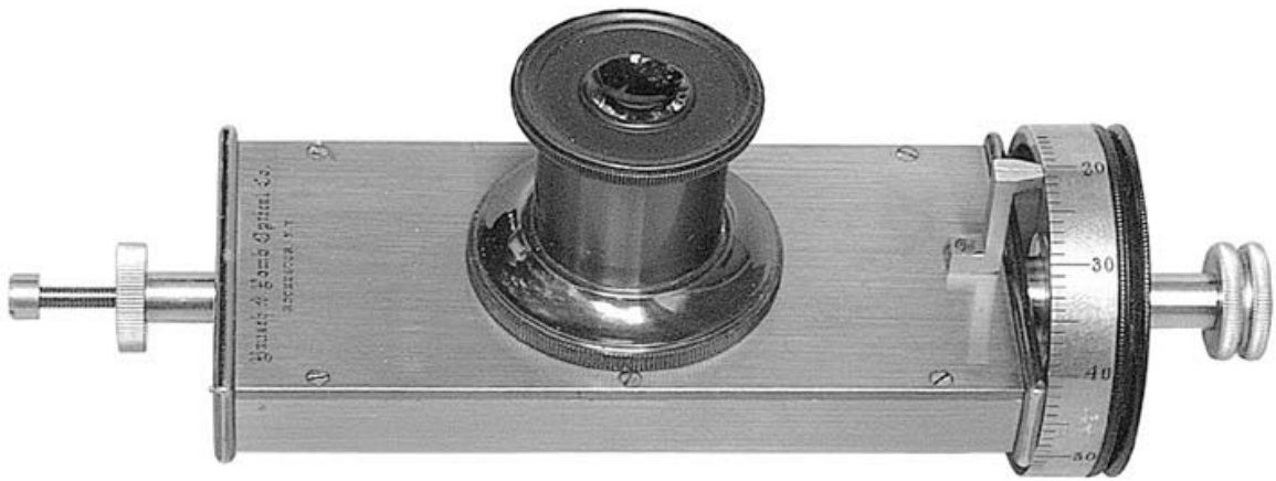
B&L Filar Micrometer, c.1900, A.Bishop
