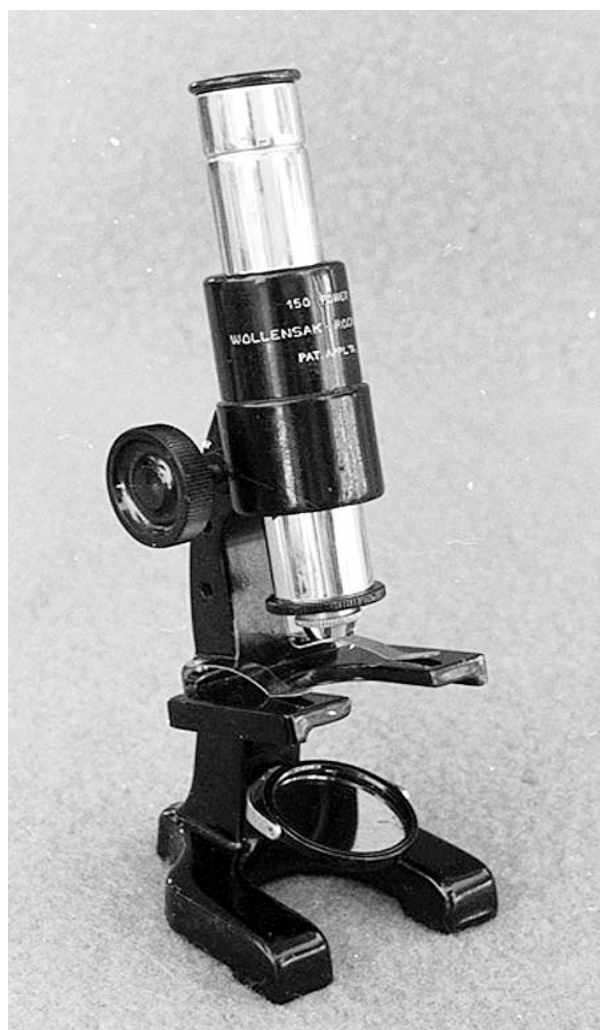
Fig. 13: The Wollensak '150 power' microscope with the draw tube retracted. Magnification is 70x.
