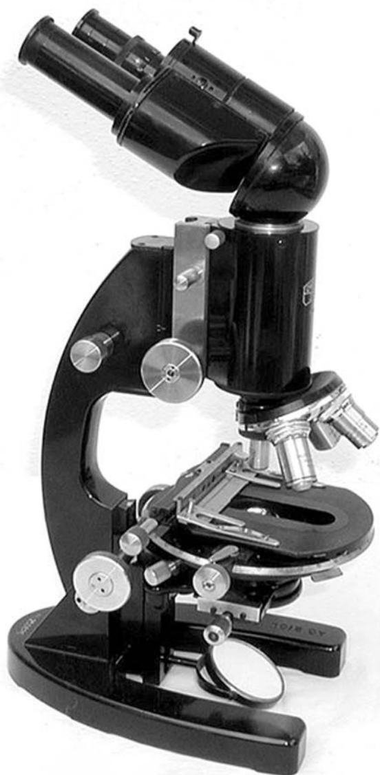
Zeiss "S" Model (Final version) with "Butumi" binocular body ca. 1938 Exhibit by Ken Gregory
