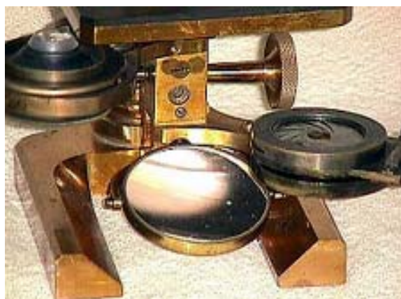
Fig. 4 Substage of the First Prize Schrauer microscope of 1894. Note the independent movement of the condenser and iris diaphragm.
