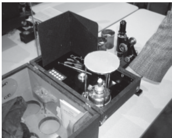
1930s Spencer milk-testing microscope outfit including accessories and instruction booklet
